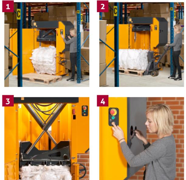
**1** Compact your waste and eject the finished bale. **2** Remove and store the bale until collection. **3** The cross cylinders ensure stable compression and a low overall height. **4** The bale is ejected by a safe two-hand operation.
